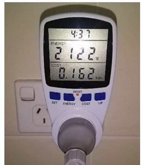
A plug-in power meter
