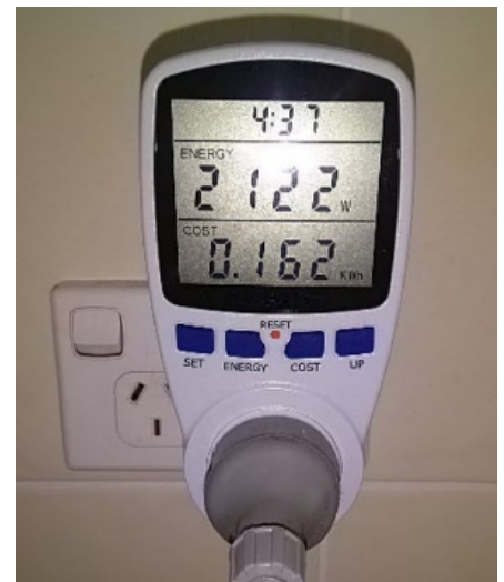
A plug-in power meter
